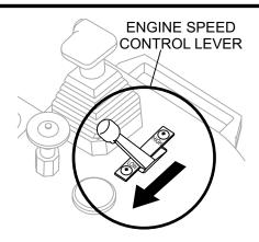
Figure 9. Engine Speed Control Lever (Low)
